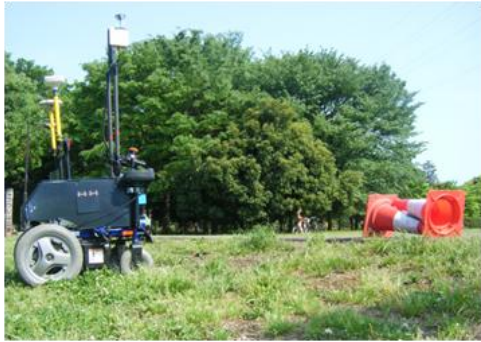
Fig.4 Obstacle detection by 2 LRFs
